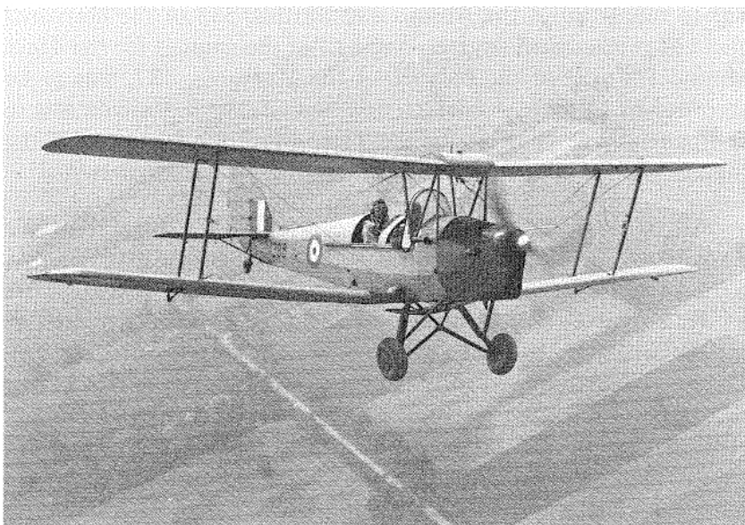
A deHavilland Tiger Moth in flight. Produced in Canada, the Tiger Moth was the most widely used elementary trainer and most of the pilots who were trained in 1940, 1941 and 1942 took their first flights in these machines. A total of 1,384 were delivered to the RCAF plus another 136 designed to take the American Monasco engine in place of the British Gipsy Major. (PI, 3582)
