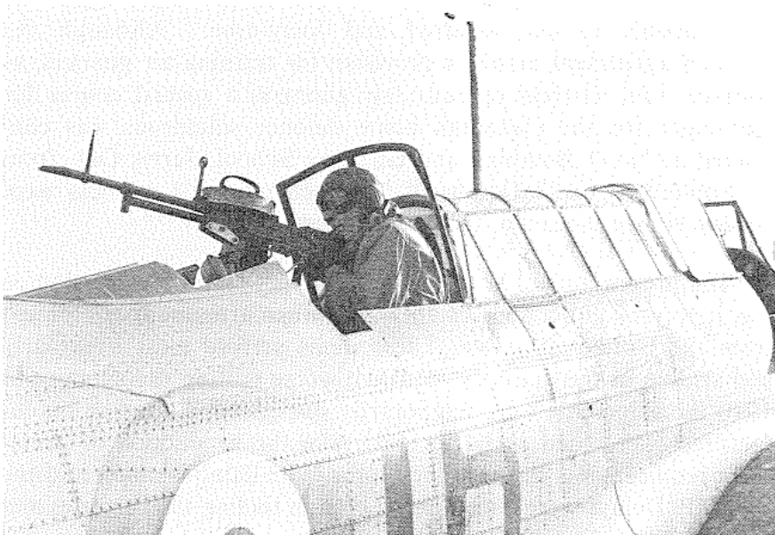
Fairey Battles were used at Bombing and Gunnery Schools for gunnery training and also for target towing. On many of these aircraft the obsolete open cockpit gun mounting was replaced by modern electrically operated gun turrets. The weapon in the photograph is a Vickers "K" gun. (PL 964)
